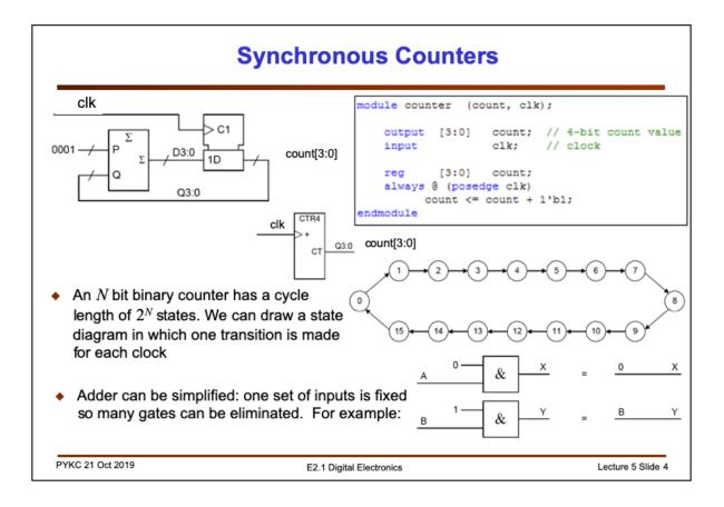
Here is the design of a 4-bit synchronous counter in schematic form. The four D-FFs store the current count value. The adder is used to compute the next count value and fed to the input of the D-FFs. On every positive edge of the signal **clk**, the count value **count[3:0**] goes up by one.
