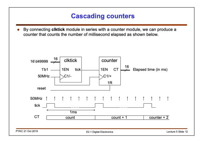
Using this style of designing a clock tick circuit allows us to easily connect multiple counters in series as shown here.
