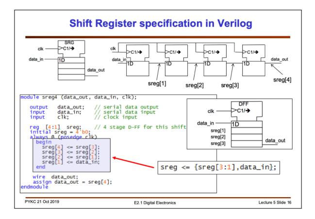
To specify a shift register in Verilog, use the code shown here (in blue box). We use the <= assignment to make sure that **sreg[4:1]** are updated only at the end of the **always** block.
