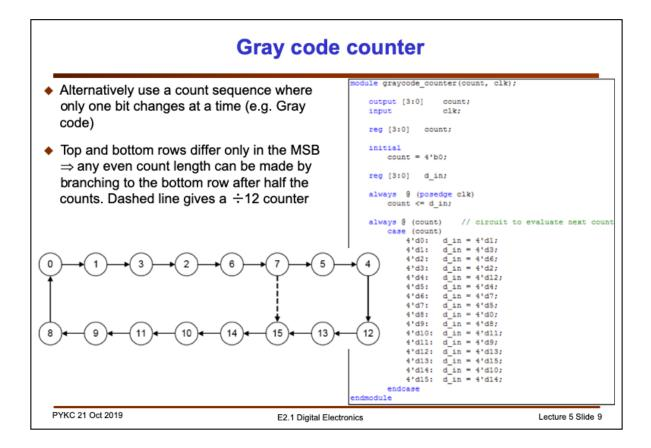
If the one-cycle delay is not desirable and you need to avoid any glitches, one could use a special counter that counts in a special sequence that guarantees NOT to produce glitches when its count outputs are gated together. The count sequence is known as Gray code.
