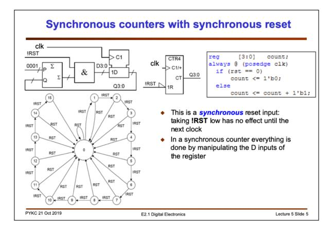
Here is a modification from the previous counter by adding a low-active reset signal **RST** (shown as !RST).
