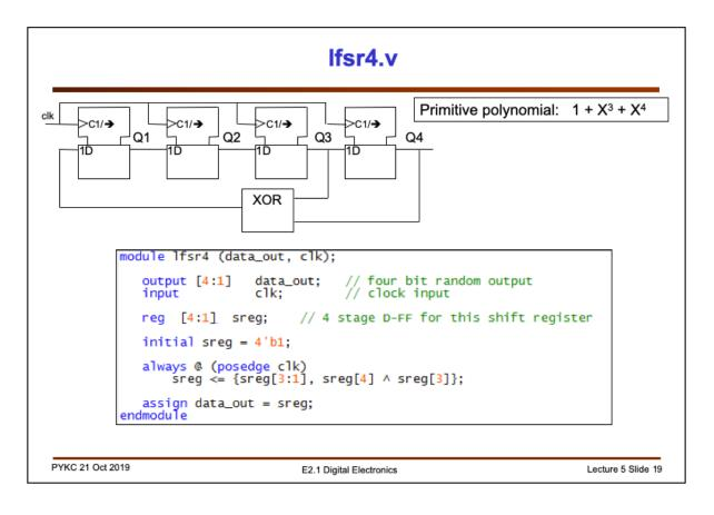
Here is the Verilog specification for a 4-bit LFSR. Note how the concatenation operator is used in the always block.
