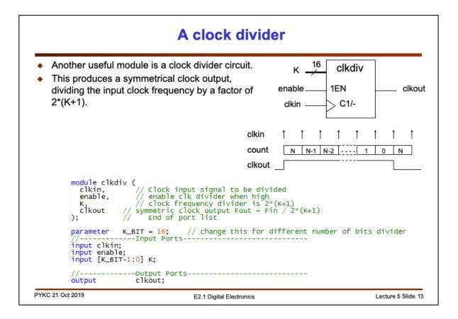
Here is yet another useful form of a counter. I call this a *clock divider*. Unlike the **clktick** module, which produces a one cycle tick signal every N+1 cycle of the clock, this produces a symmetric clock output **clkout** at a frequency which is the input clock frequency divided by 2\*(K+1).
