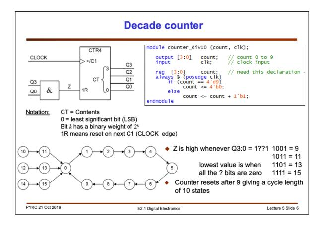
What if you want a counter that only counts from 0 to 9, then back to 0 again? This is really easy with Verilog. A simple if-else construct testing for the terminal counter of 9 will do the trick.
