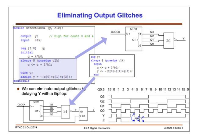
Eliminating glitches can be achieved by adding an extra D-FF at Y output. Z will be glitch free. However, **beware that Z is one cycle delayed relative to Y**.
