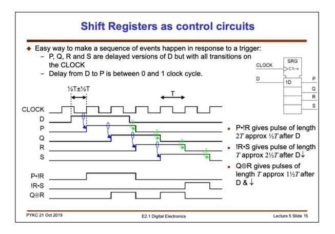
Instead of producing binary signals using a counter, one could use a shift register to produce a sequence of pulses delayed relative to each other, and use gates to merge these together and produce different binary signals.
